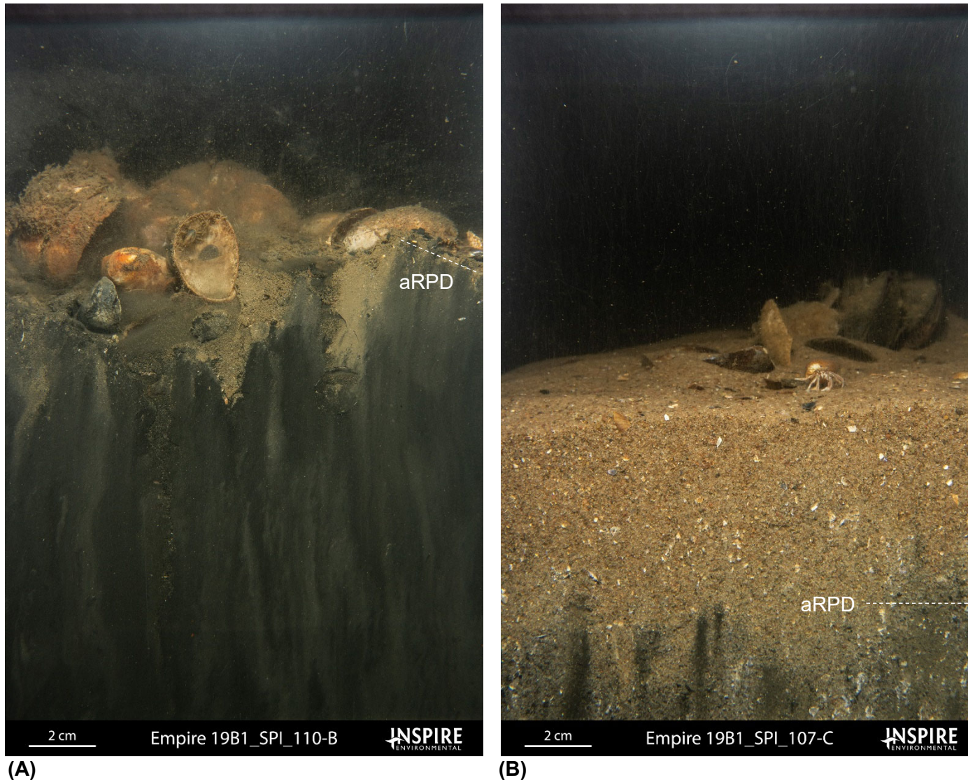
Figure 3-58. Profile images depicting (A) Station 110 with a diffusional aRPD and high sediment oxygen demand (SOD), note oxid brown sediment is dragged down into sediment column; and (B) Station 107 with a deep aRPD and medium SOD. Stations 110 and 107 had the shallowest and deepest aRPDs, respectively, along the New York Harbor Export Cable Route.
